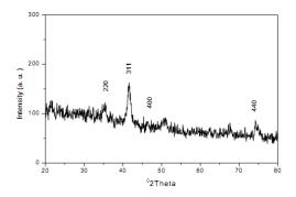
Figure 1. XRD spectrum of iron oxide nanoparticles [Fe<sub>3</sub>0<sub>4</sub>]: using Debye-Scherrer method, particles sizes were calculated 15-20 nm.
