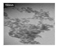
Fig 2. TEM image showed that the nanoparticles had average diameters of 10-15 nm.
